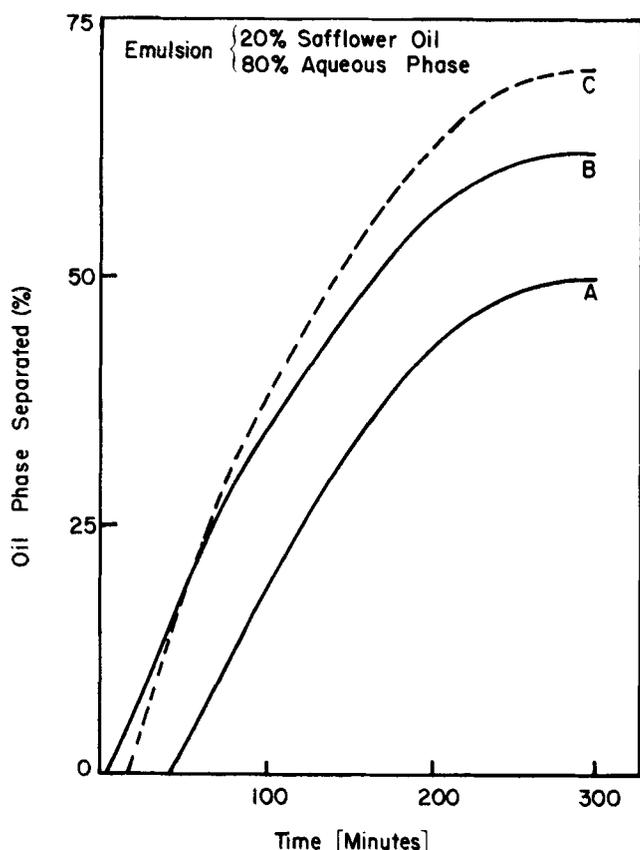
FIG. 7. Emulsion stability from volume of oil expelled vs. time. A = No HCl; B = 1 ml.; C = 1.4 ml. of 0.1N HCl.
