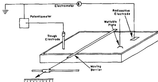
FIG. 3. Schematic Diagram of Film Balance.
