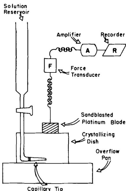
FIG. 2. Apparatus for determining dynamic surface tensions.
