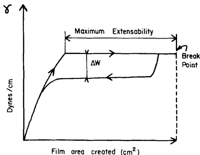
FIG. 5. Typical tensiolaminometry results.
